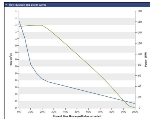
**Figure 9.** Power Output – Sg. Tebing Tinggi MHP (Existing)
