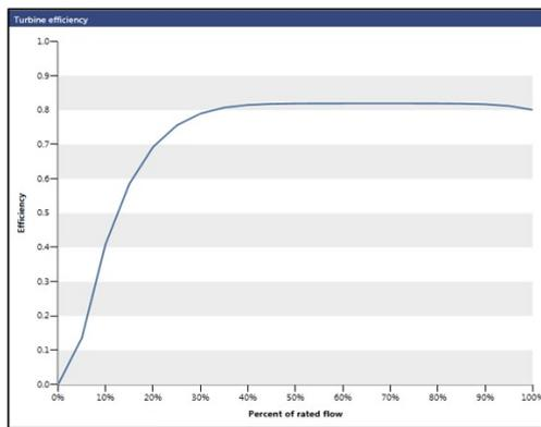
**Figure 8.** Turbine Efficiency Curve – Sg. Tebing Tinggi
