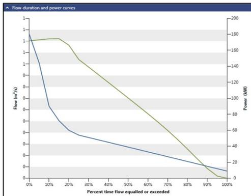
Figure 10. Power Output – Sg. Tebing Tinggi (New)
