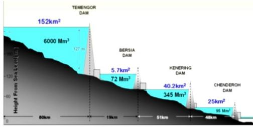
**Figure 1.** Advisable DAM Operations in Sg Perak Hydroelectric Scheme
