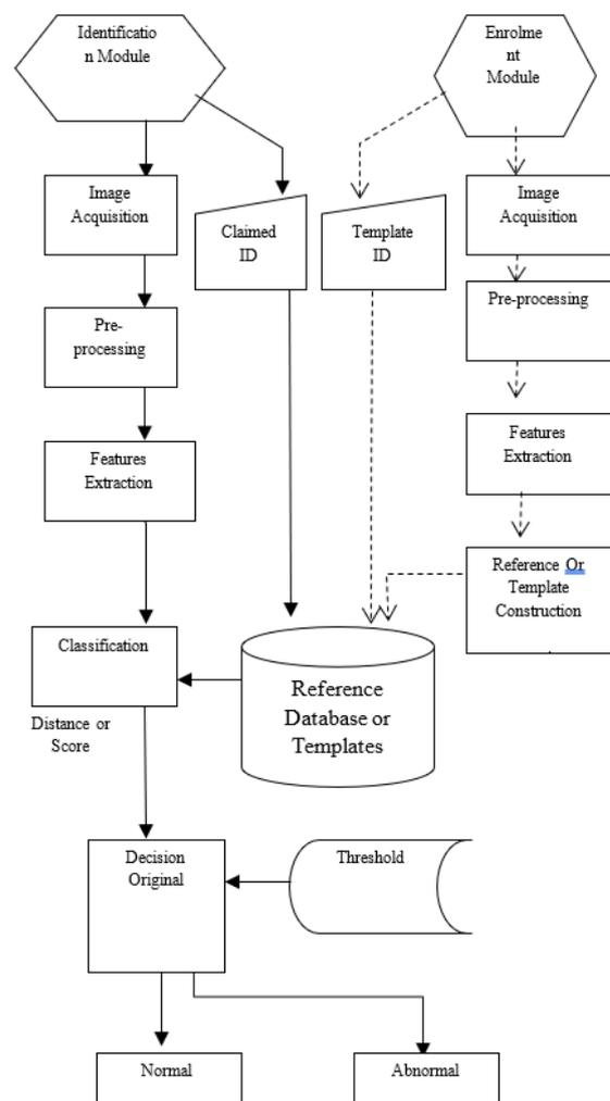
**Figure 2.** Block Diagram of the Proposed ECG identification System
