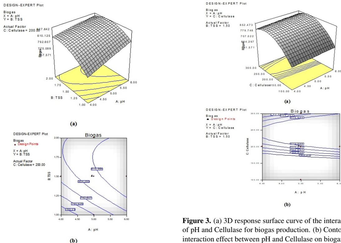
**Figure 3.** (a) 3D response surface curve of the interaction effects of pH and Cellulase for biogas production. (b) Contour plot of interaction effect between pH and Cellulase on biogas production**Figure 2.** (a) 3D response surface plot for the optimization of biogas production based on pH and Total Suspended Solids (TSS) ; (b) Contour plot of interaction effect between pH and TSS on biogas production
