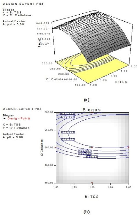
**Figure 4.** (a) 3D response surface curve of the interaction effects of TSS and Cellulase for biogas production. (b) Contour plot of interaction effect between TSS and Cellulase on biogas production
